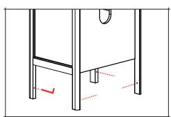
Console units (SO060C) can be levelled with an allen key.
