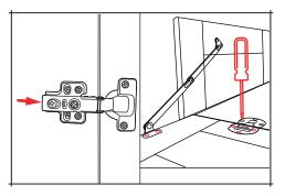
Before mounting the unit, we recommend fitting the handles. To do this, simply press the button at the back of the hinge. The entire door and hinges will release from the carcass. For units with a top panel, unscrew the hinges and guides from the panel to remove the panel.
